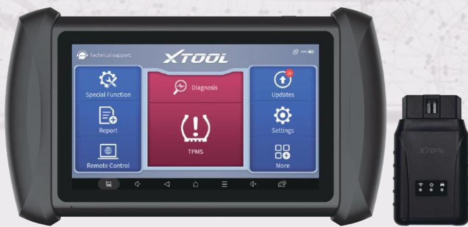
InPlus IP819 TP is an automotive TPMS diagnostic system with a 7-inch LCD display, integrated Android OS and highly-customized diagnosis interface.
